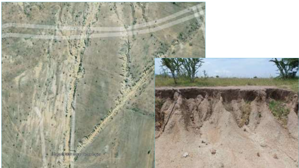
Figure 6-8: Main picture: straight excavated drains that have eroded and incised to become deep, broad, highly eroded gullies (Image from Google EarthTM, 2004). Inset: Estcourt soil form, showing distinctive difference between the shallow sandy topsoil and the hardened, erodible subsoil of Prismaeutanic clay
