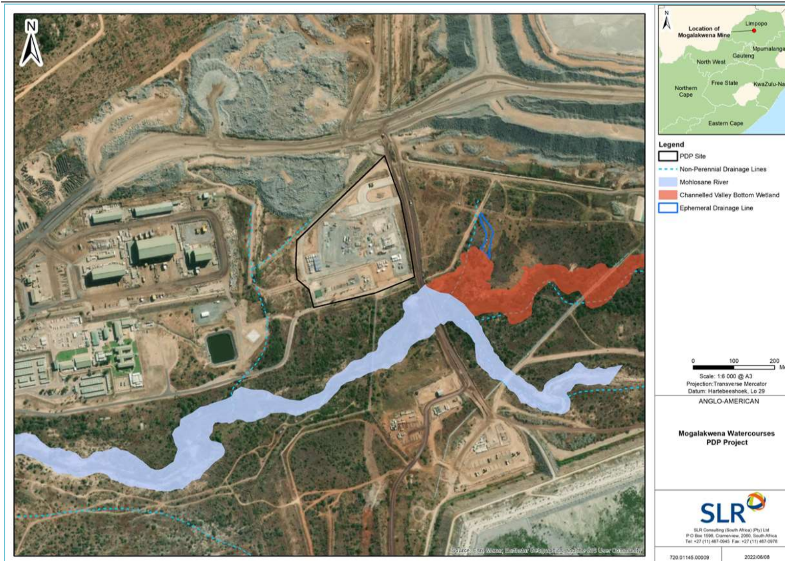
Figure 6-4: Local Drainage context of the Project area
