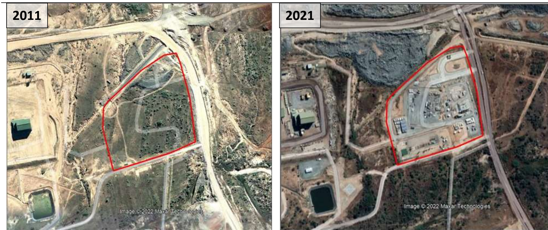
Figure 6-2: Google Earth™ satellite imagery showing the timescale of the disturbance at the site. The image on the left is from 2011, and indicates historic cultivation, the complete removal of primary vegetation and a degree of soil sheet erosion; the image on the right is from 2021 and shows existing mining infrastructure.
