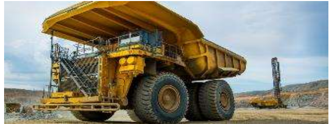
Dilori tša Haul tša Go Sepelela ka Hydrogen (Difatanaga tša Disele tša Makhura a Mohlagase (Fuel Cell Electric Vehicle (FCEV)) 2
