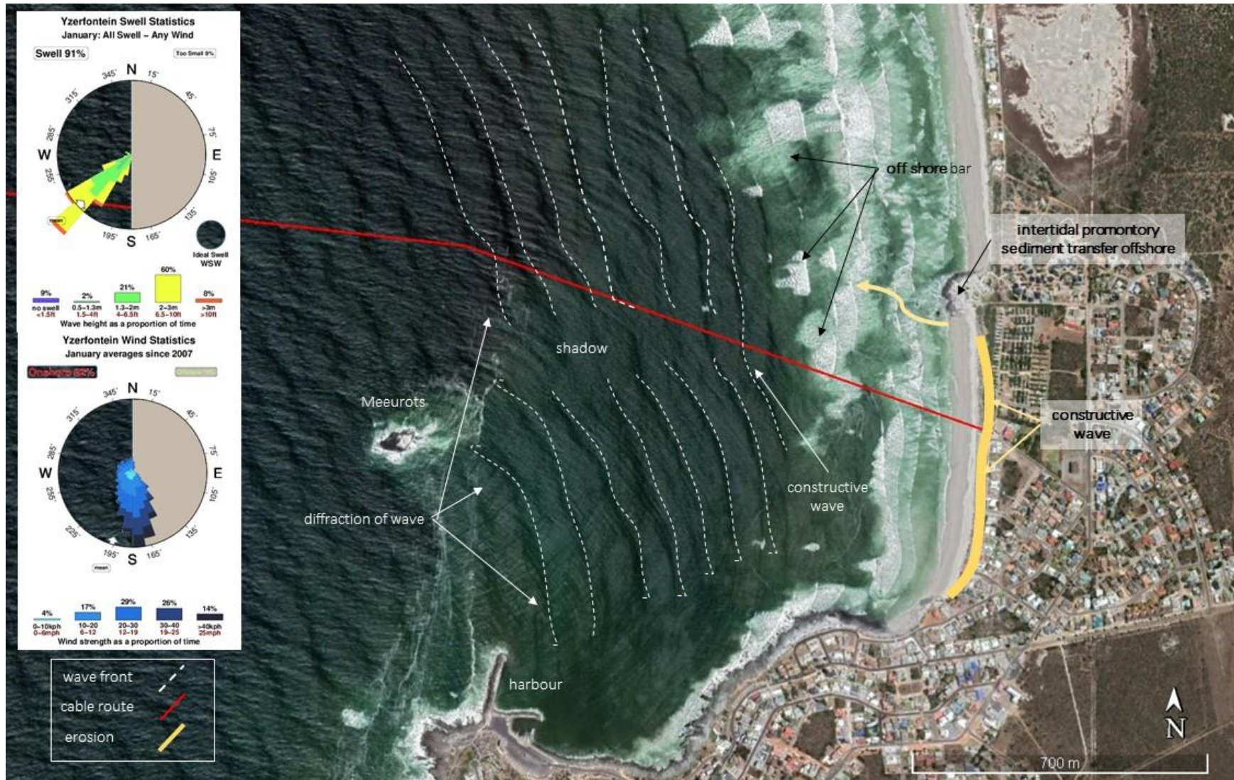
Figure 7. Aerial photograph showing features and coastal dynamics at site of cable landing, Yzerfontein.
