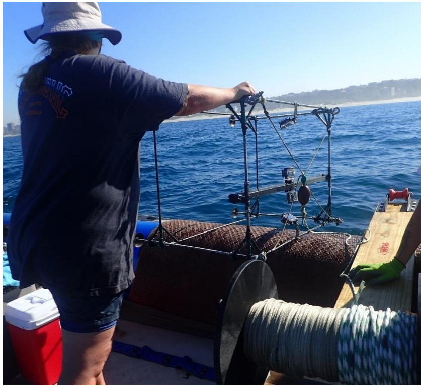
Figure 3.1: The drop camera system used for the marine benthic assessment along the Amanzimtoti Pipeline Beach Landing Site.
