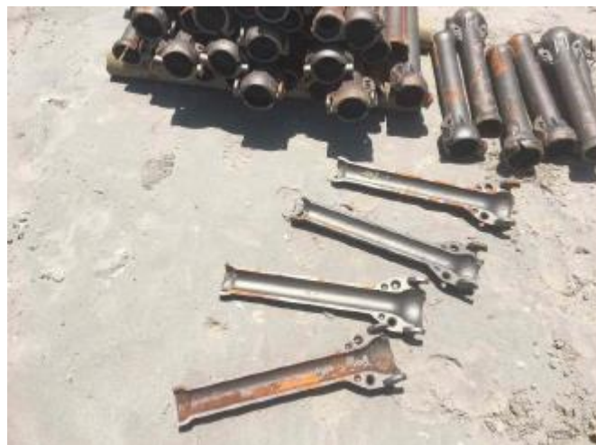
Figure 2.2: Articulated split pipe used for cable protection in the shallow inshore regions. The pipe ranges in diameter from 55mm at the narrowest end to 148mm at the coupling.
