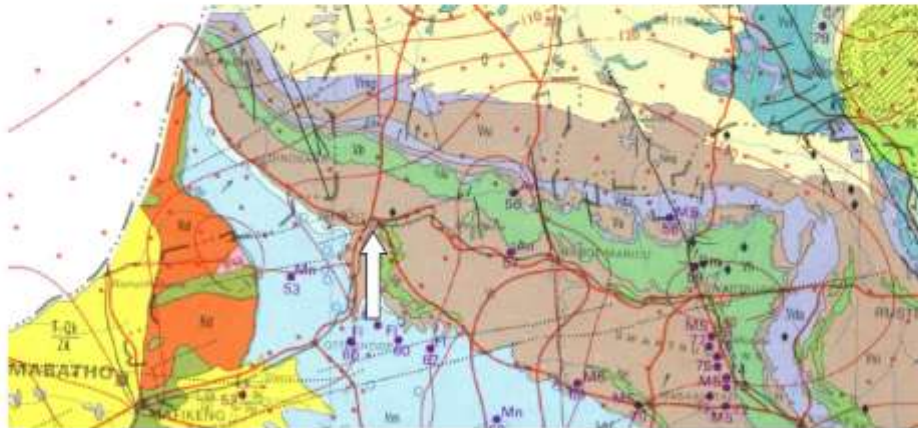
Fig 1: Geology of the region around Zeerust and locality marked with white arrow. Map enlarged from the Geological Survey, Pretoria; 1984, 1: 1 000 000. Vt = Timeball Hill and Rooihoogte Formations (Pretoria Group); Vdi = Vaalian, diabase.
