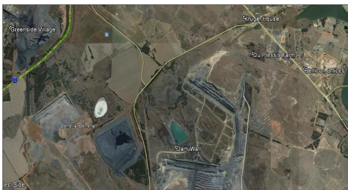
Figure 65: Ground Vibration and Air Blast monitoring locations (source: Blast Management and Consultin, September 2016))
