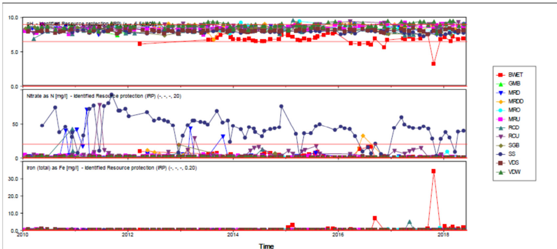
Figure 13: pH, nitrate and total iron variation in river samples
