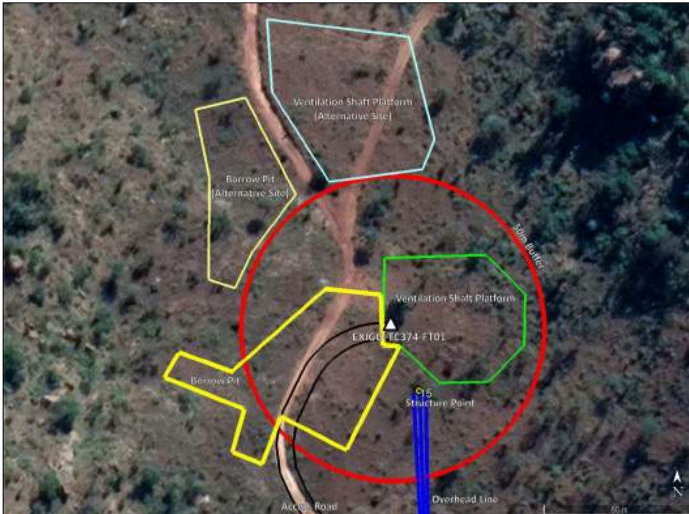
Figure 6-8: Aerial map indicating recommended mitigation measures and possible alternative positions for infrastructure around Site EXIGO-TC374-FT01 and the required conservation buffer.
