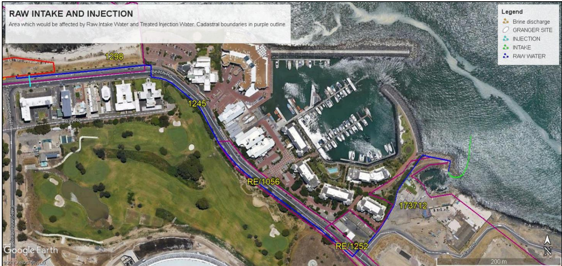
Figure 1.7: Proposed raw water abstraction infrastructure in context. (Source: Google Earth 2010-01-08 imagery).
