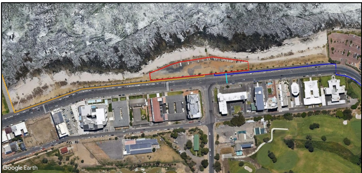
Figure 5.3.1: Proposed site and incoming and outgoing pipelines in local context 2010 Site indicated in red outline; dark blue line indicates incoming raw water pipeline; light blue line indicates treated water injection pipeline; and orange line indicates brine discharge pipeline (Source: Google Earth 2010-08-01 imagery).
