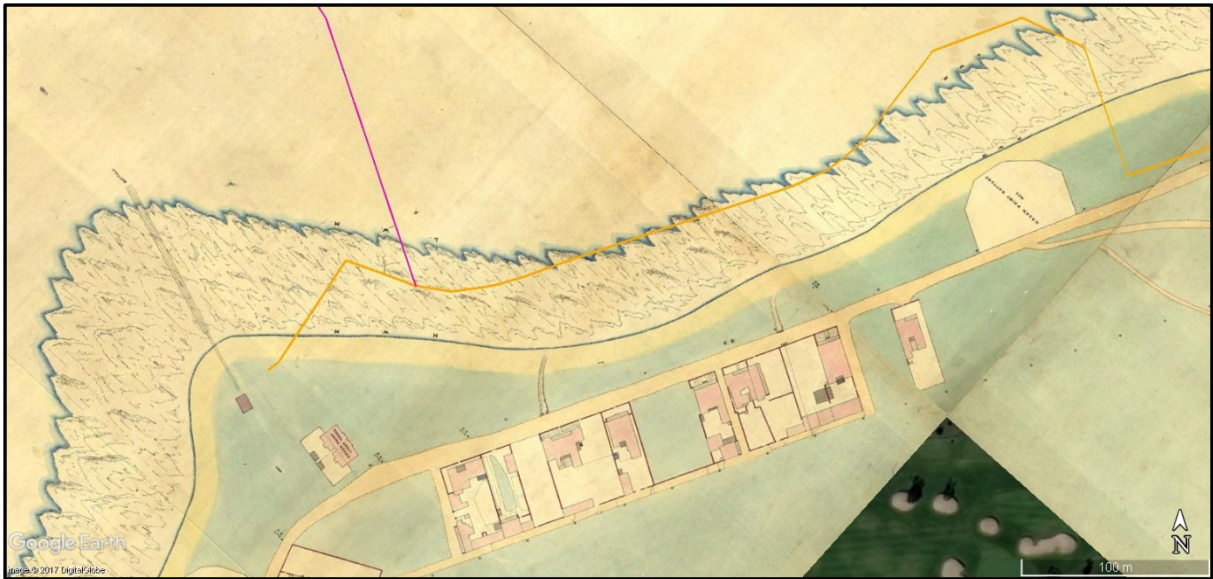
Figure 5.2.2: Terminal portion of brine discharge pipeline (orange line) and existing outfall (pink line) in local context ca 1900. (Source: Walter Thom Survey, Sheets 116; 123; and 124).
