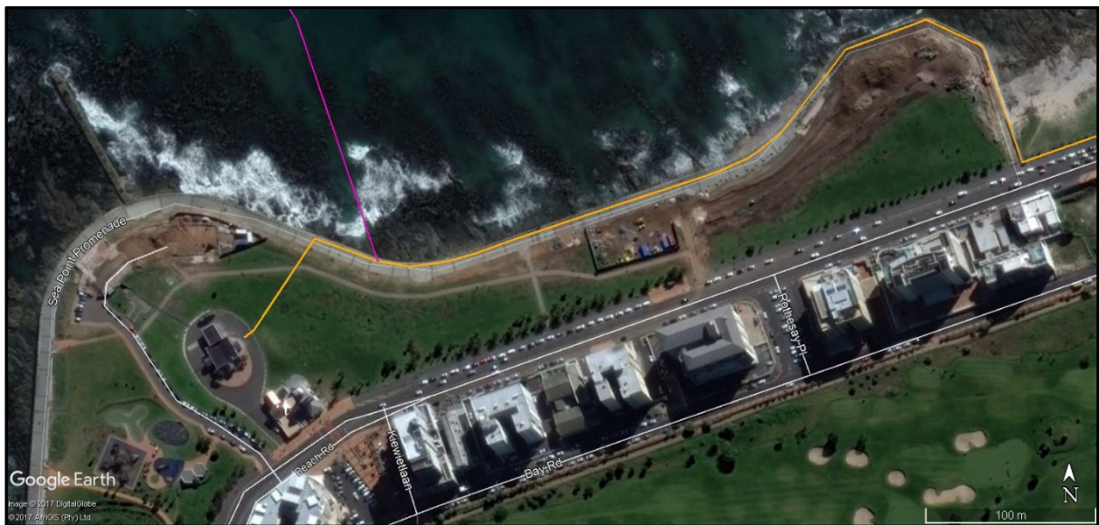
Figure 5.2.1: Terminal portion of brine discharge pipeline (orange line) and existing outfall (pink line) in local context 2017. (Source: Google Earth 2017-08-26 imagery).
