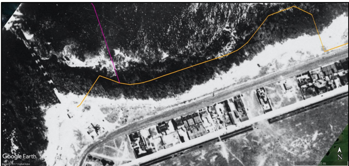
Figure 5.2.3: Terminal portion of brine discharge pipeline (orange line) and existing outfall (pink line) in local context 1926. (Source: Chief Directorate: National Geo-spatial Information 1926_2_831).
