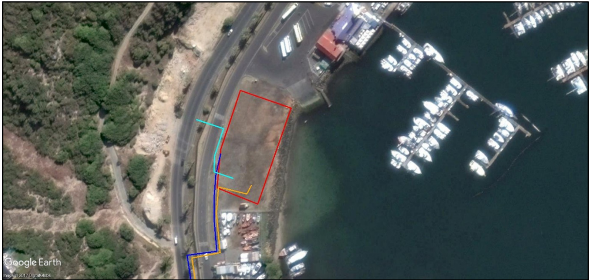
Figure 5.2.1: Hout Bay desalination plant site, incoming raw water pipeline, and outgoing treated water injection and brine discharge pipelines in local context 2017. (Source: Google Earth, 2017-05-12).
