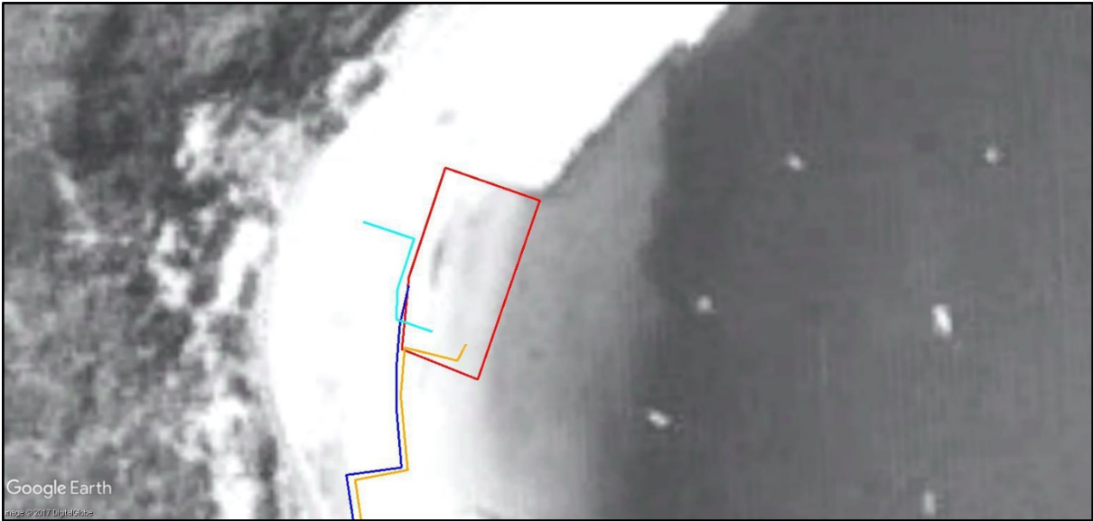
Figure 5.2.5: Hout Bay desalination plant site, incoming raw water pipeline, and outgoing treated water injection and brine discharge pipelines in local context 1968. (Source: Chief Directorate National Geo-spatial Information. 620/68_2_265).
