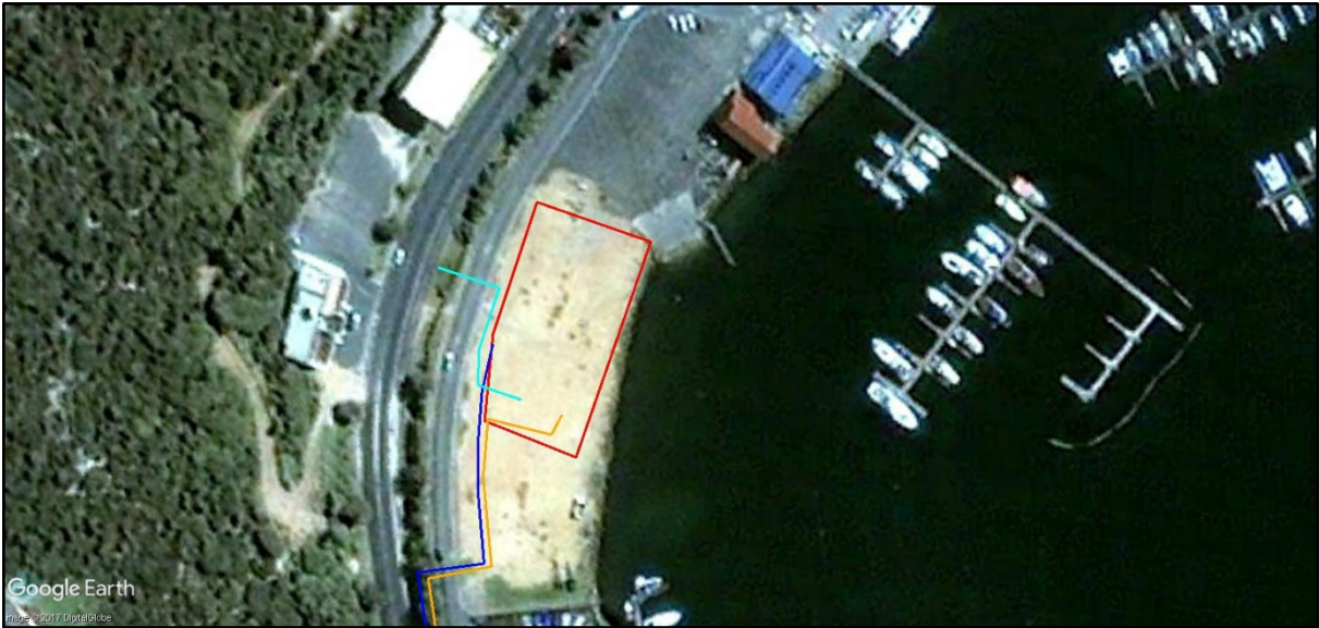
Figure 5.2.7: Hout Bay desalination plant site, incoming raw water pipeline, and outgoing treated water injection and brine discharge pipelines in local context 2001. (Source: Google Earth, 2001-09-14).
