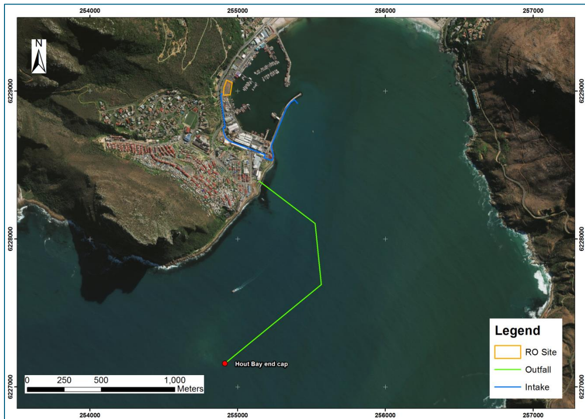
Figure 1-1: Hout Bay desalination plant option.
