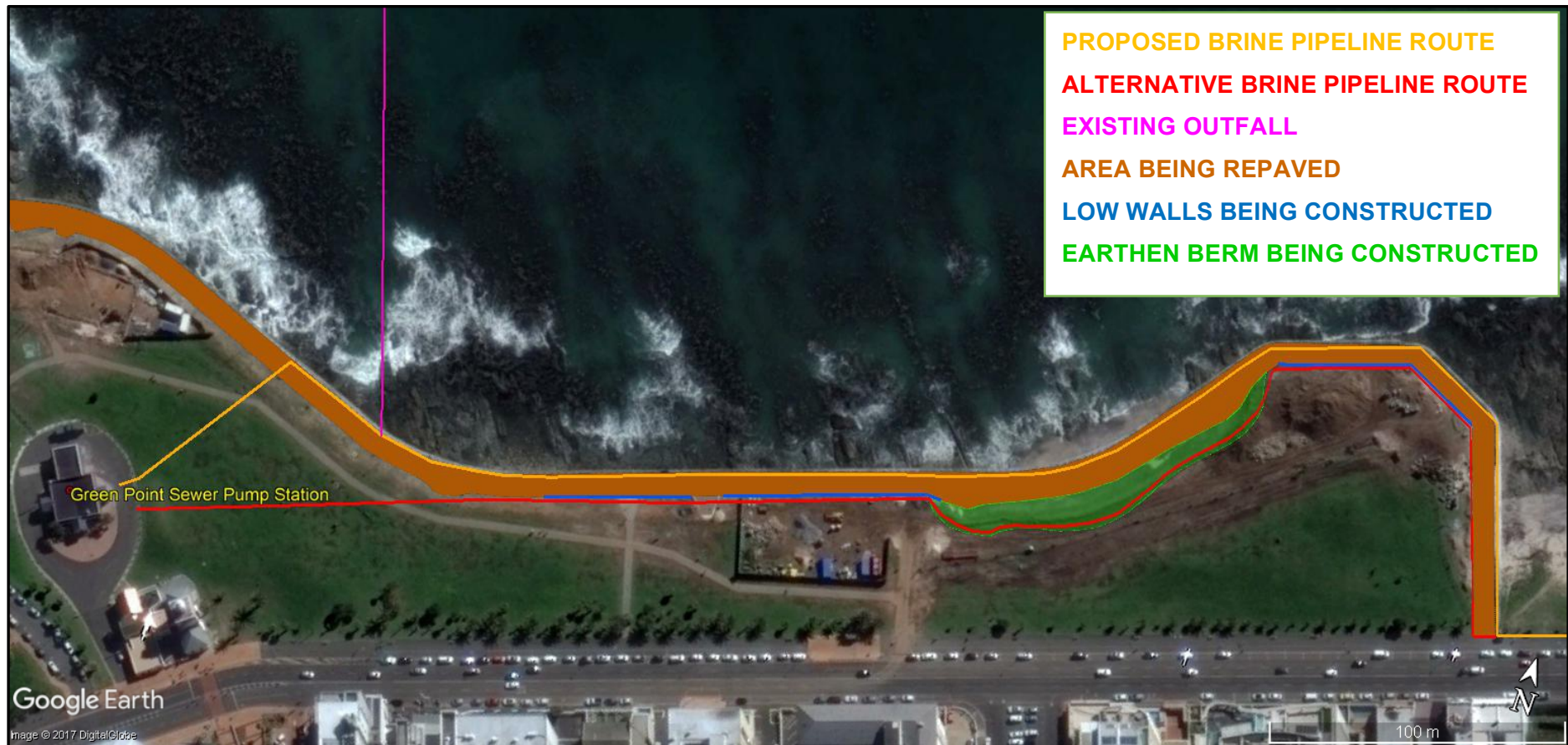
Figure 8.2. Proposed Alternative (Mitigation) Brine Discharge Pipeline route in relation to proposed route (Project) and landscaping upgrades currently being undertaken along this portion of the Promenade.
