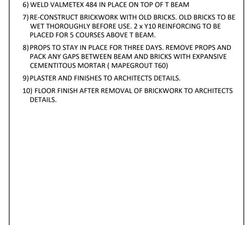
**INSTALLATION OF STEEL T BEAM** 1) NEATLY REMOVE EXISTING BRICKS, ABOVE NEW T BEAM. REMOVE PLASTER AND MORTAR AND STACK FOR RE-USE.
