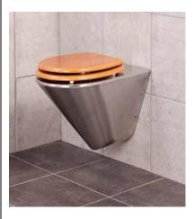
**Paraplegic toilet pan** - Manufactured from Grade 304 (18/10) Stainless Steel, 360 x 700 x 350 mm. Unit to be a back entry or a top entry (please specify product code when requesting quotes). Unit to be supplied with 3 mm thick Stainless Steel wall fixing bracket and fitted in accordance with manufacturers specifications using 4 x 8 mm anchor bolts (measured separately). Compliant with SABS 1733:1998 and SABS 497:1991.
