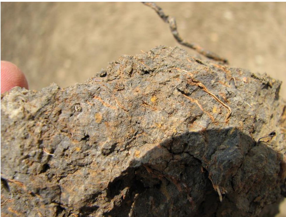
Figure 18: Orange rhizospheres and orange mottles within a gleyed grey reduced matrix sampled within a low-lying area of a hillslope seepage wetland
