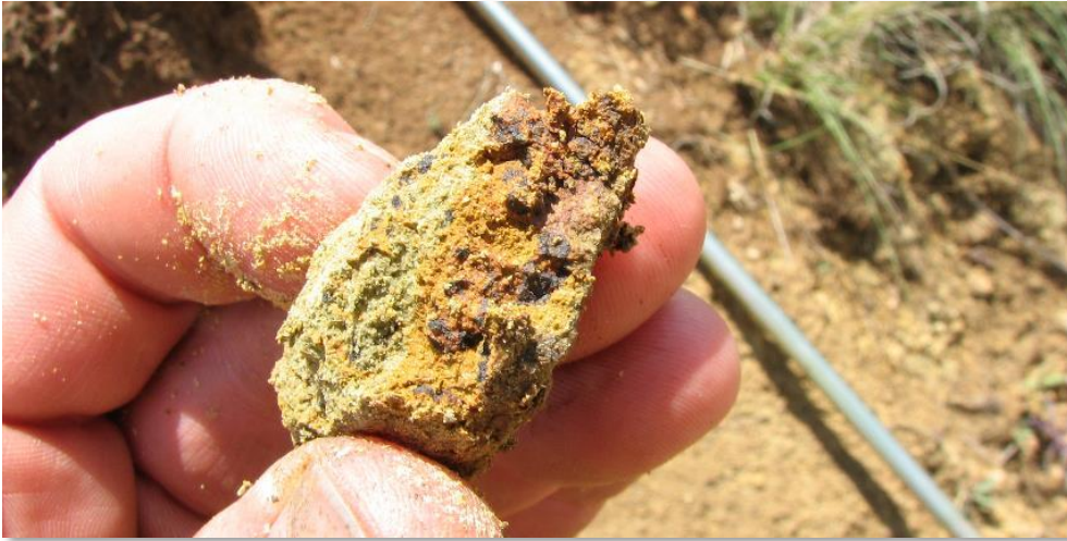
Figure 17: Augered sample of plinthic horizon with black mottles likely to be manganese
