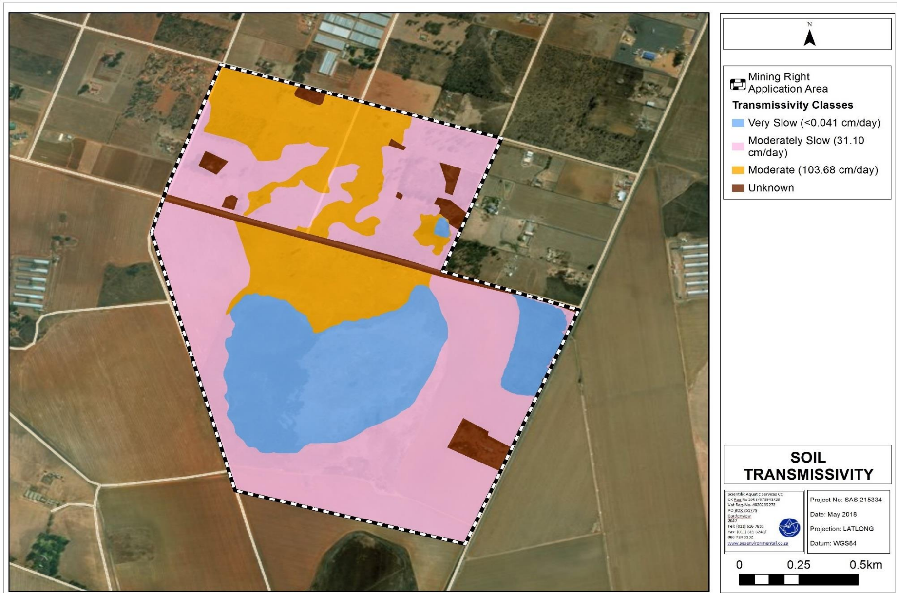
Figure 18: A map depicting soil transmissivity of the representative soil samples across the investigated wetland catchment.
