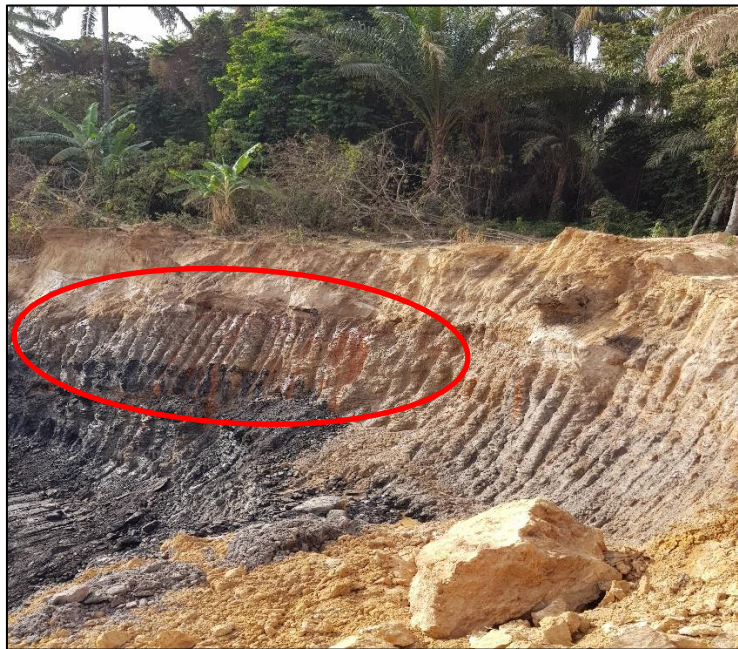
Figure 19: An example of interflow in the subsoil indicated by the red circle
