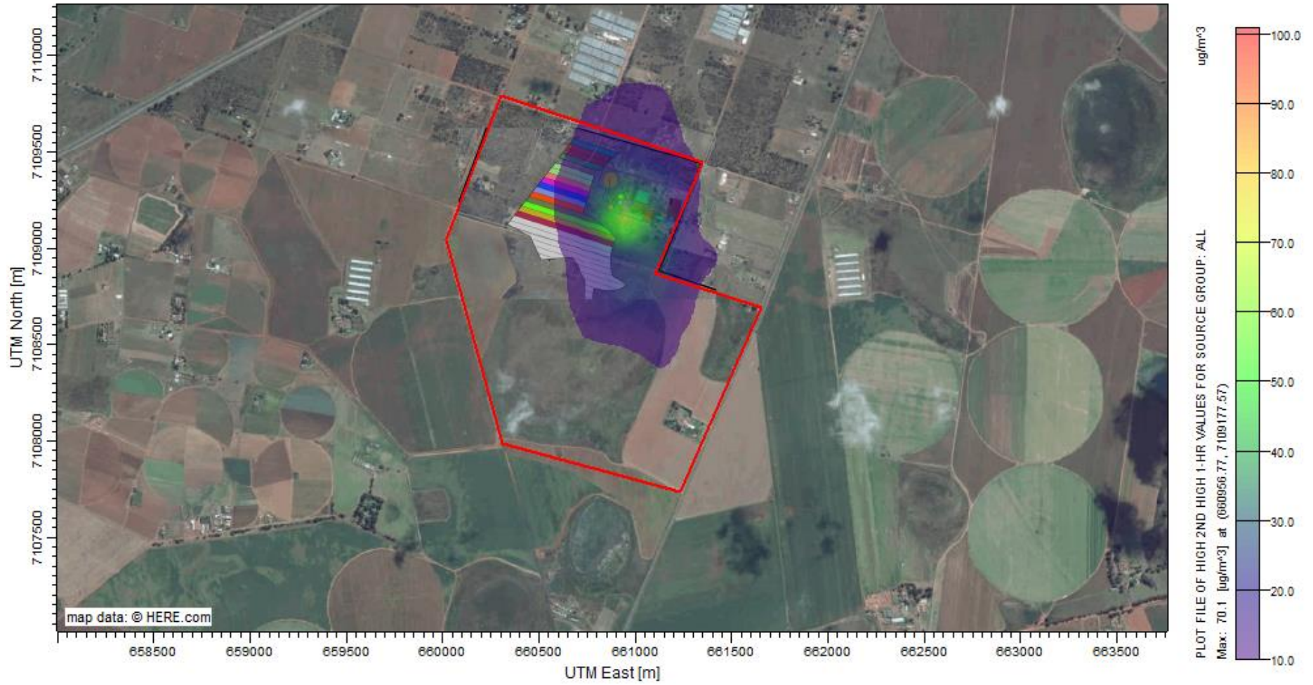
Figure 26: Hourly average predicted ambient ground level concentrations ( \mu\text{g}/\text{m}^3 ) of Sulphur dioxide (Standard: 350\mu\text{g}/\text{m}^3 )
