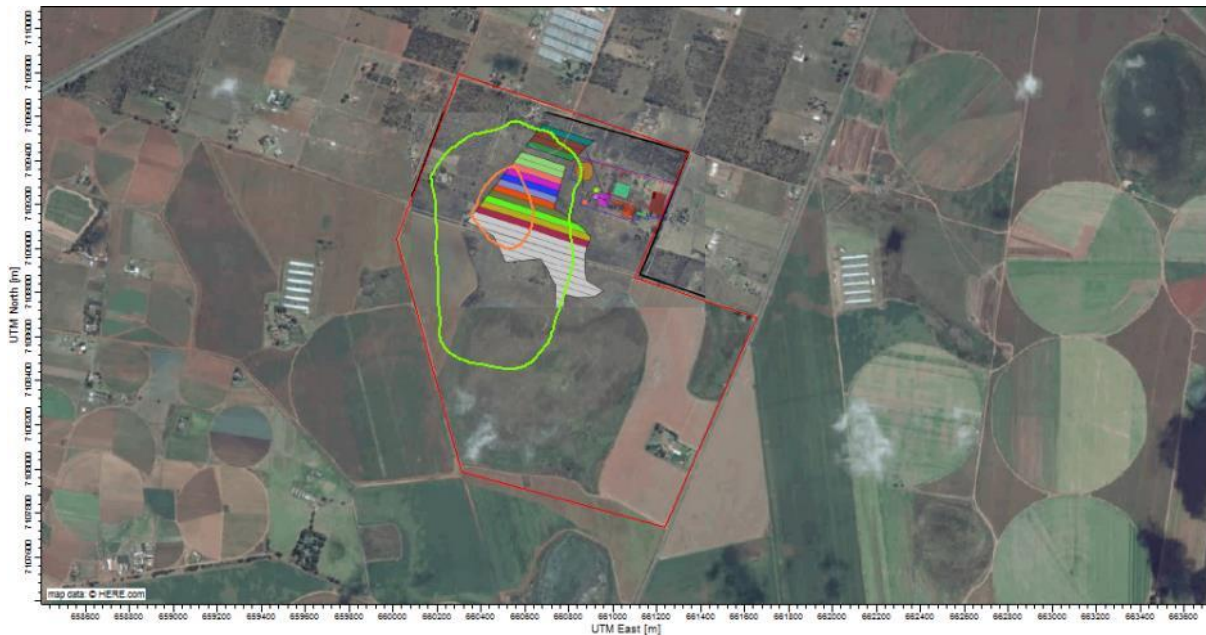
Figure 18: Predicted dust fallout impacts with the residential impact ( 600\text{mg}/\text{m}^2/\text{day} ) in green and the industrial ( 1200\text{mg}/\text{m}^2/\text{day} ) in orange
