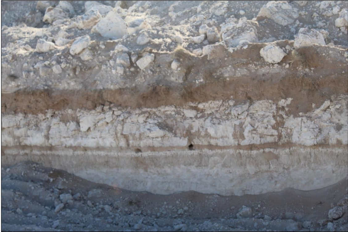
Figure 7: In the centre of the property the soil profile shows sand/silt on top and below the diatomaceous stratum
