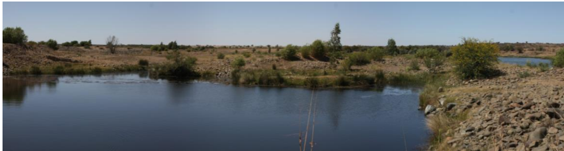
Figure 19: Mining in the upper zone has formed deep excavations which have become filled with groundwater and form artificial impoundments.
