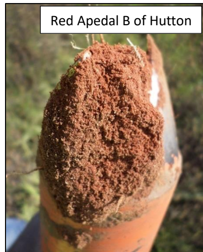
Figure 11: View of recharge soils with deep, well aerated and free draining characteristics
