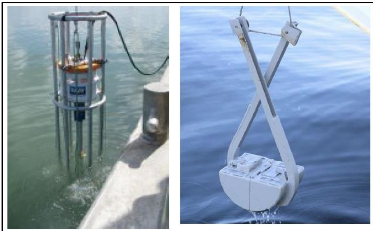
Figure 3: Left Example of a corer and right a Van Veen grab that works like a claw to grab sediment from the seafloor
