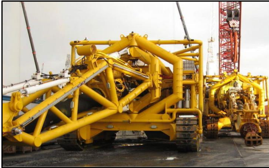
Figure 8: Example of a track-mounted sub-sea crawler
