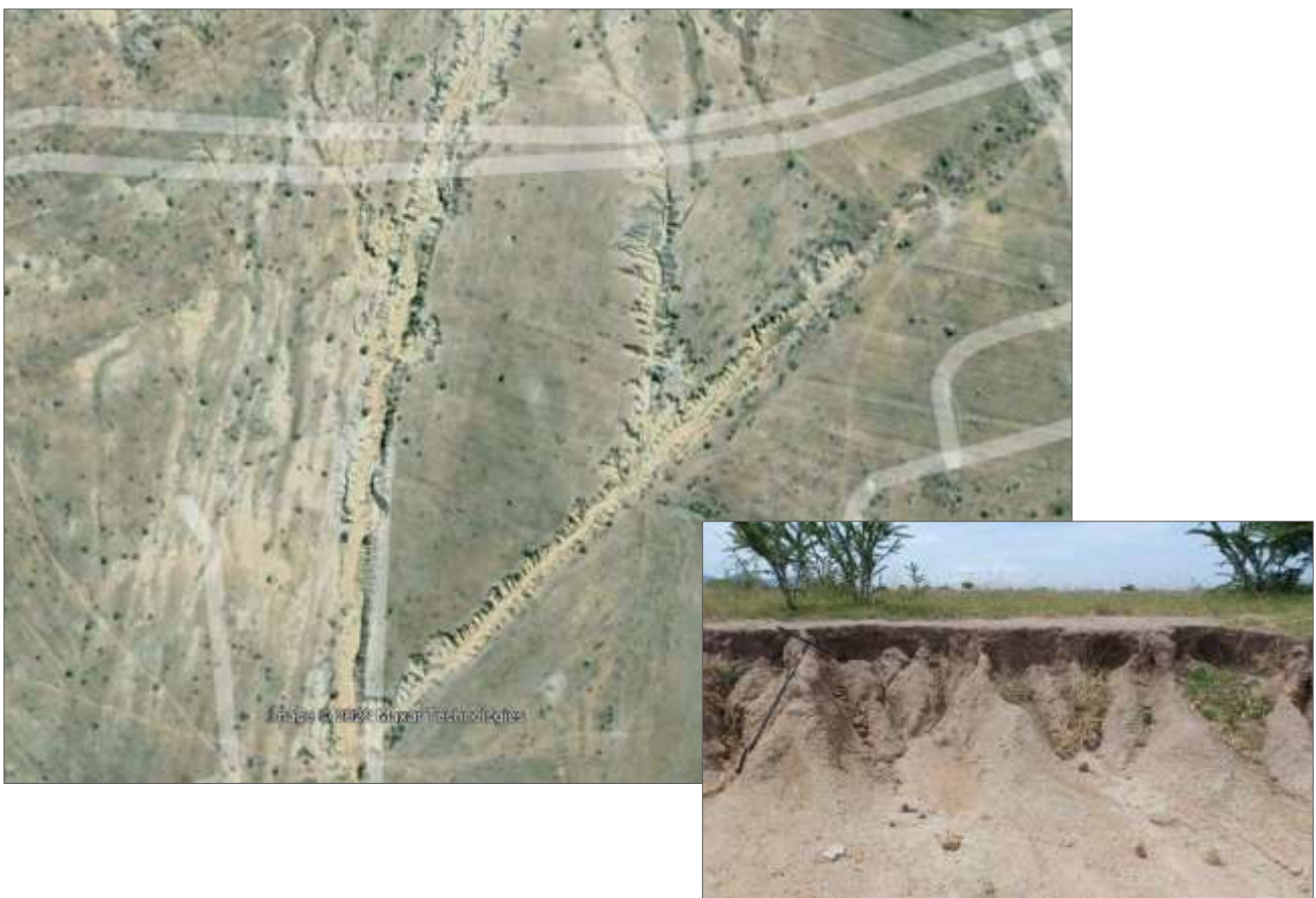
Figure 5.3: Main picture: straight excavated drains that have eroded and incised to become deep, broad, highly eroded gullies (Image from Google Earth™, 2004). Inset: Estcourt soil form, showing distinctive difference between the shallow sandy topsoil and the hardened, erodible subsoil of Prismaeutanic clay.
