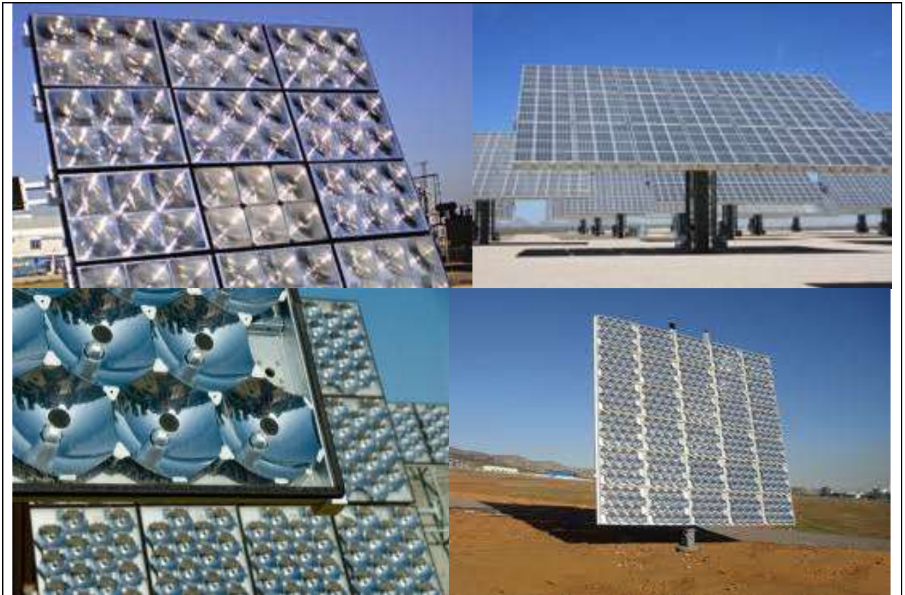
Example of Concentrated Photo-voltaic technologies (Bullis, 2011).
