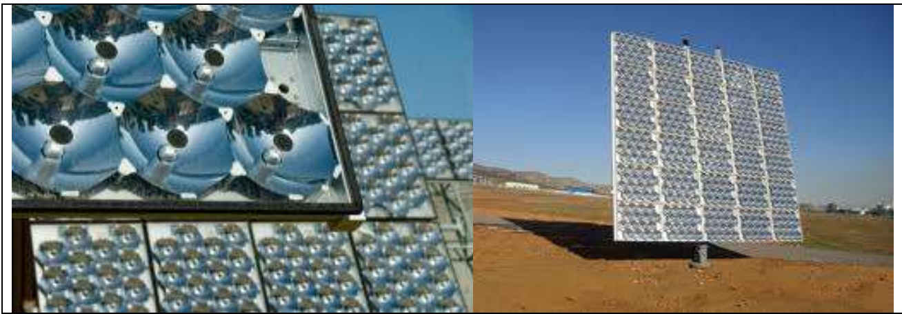
Figure 3-3: Example of Concentrated Photo-voltaic technologies (Bullis, 2011).
