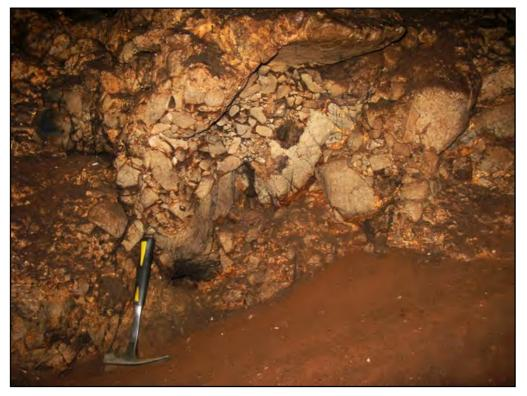
Figure 25: Reddish-brown cave earth abutting against poorly-sorted, well-cemented dolomite breccia in the SW wall of the main chamber (hammer = 30 cm). Dolomite clasts here are angular to subrounded and clast- to matrix-supported (possible debris flow origin).
