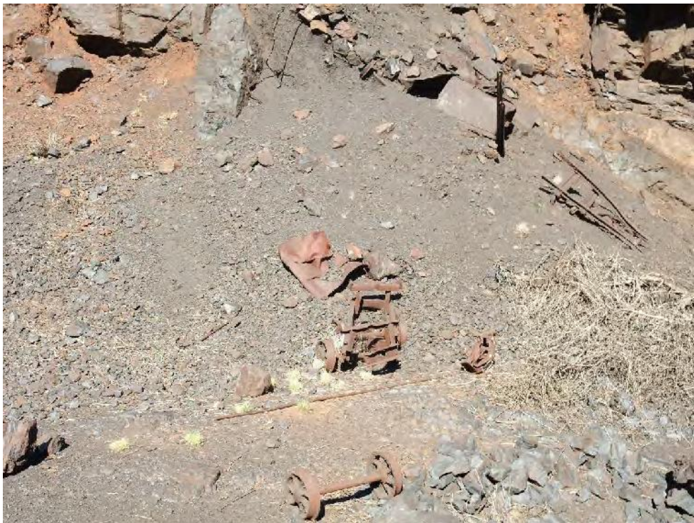
Figure 15: Undercarriage and other parts of a coco pan.
