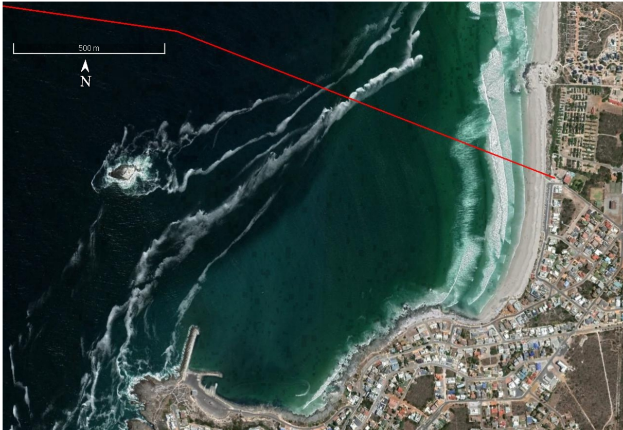
Figure 2: GoogleEarth image showing the routing of the proposed ASN 2AFRICA (West) Cable System in shallow waters and the shore crossing at the beach in Yzerfontein.
