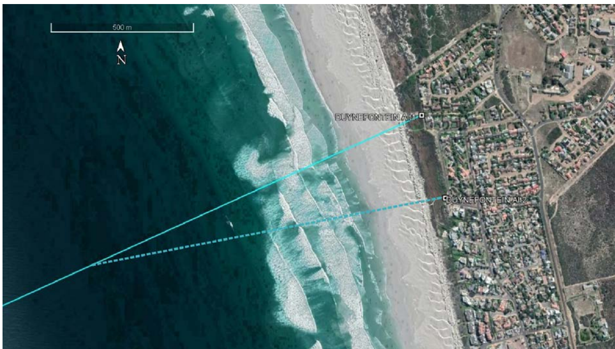
Figure 2: GoogleEarth image showing the routing of the proposed 2AFRICA/GERA (East) Cable System in shallow waters and the shore crossing alternatives at the beach in Dwynefontein.
