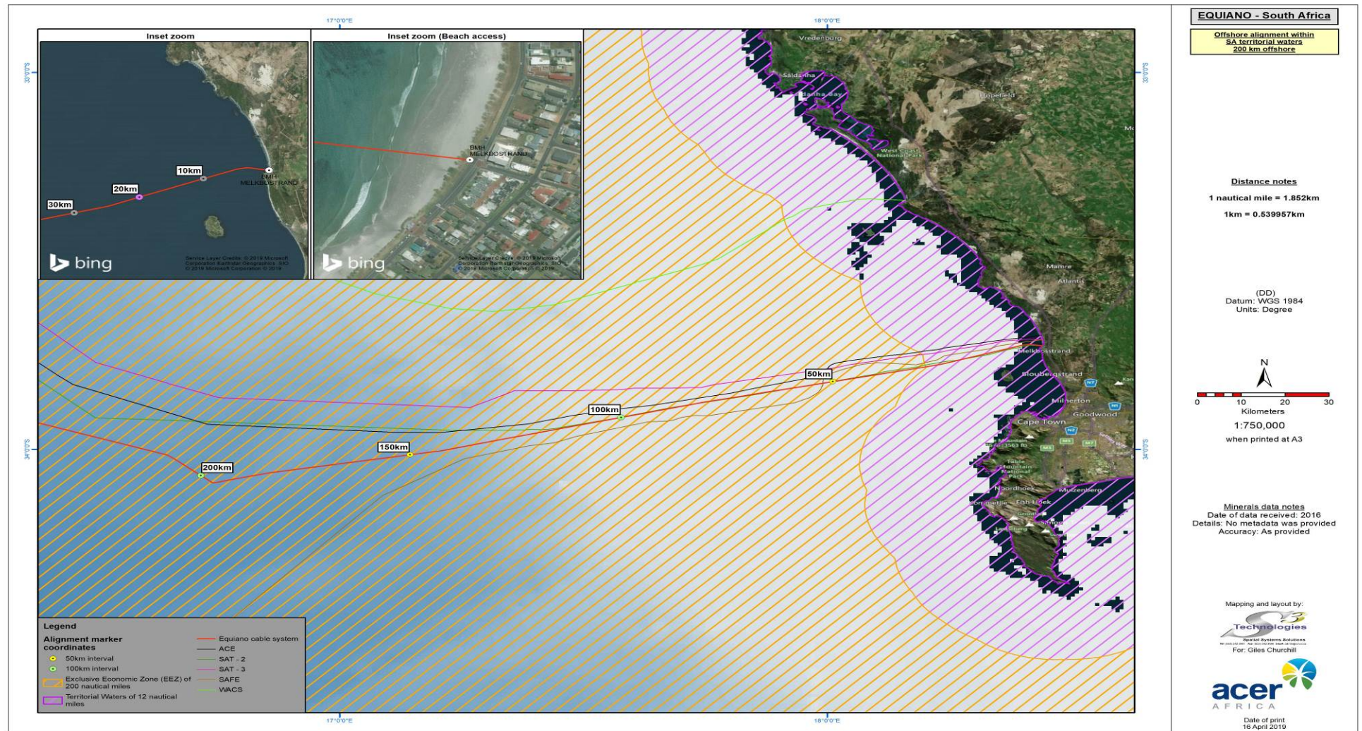
Figure 6 Alignment of the Equiano Cable System in relation to existing telecommunication cable systems landing along the Western Cape coastline
