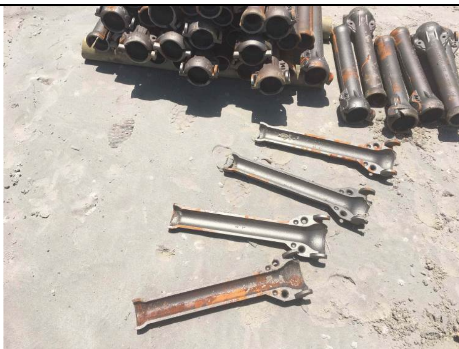
Plate 8 Articulated pipe sections which are installed around the cable in shallow water to offer additional protection.
