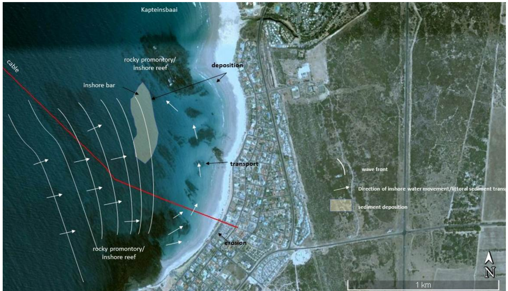
Figure 14 Graphic representation of the inshore wave and sediment dynamics at Melkbosstrand
