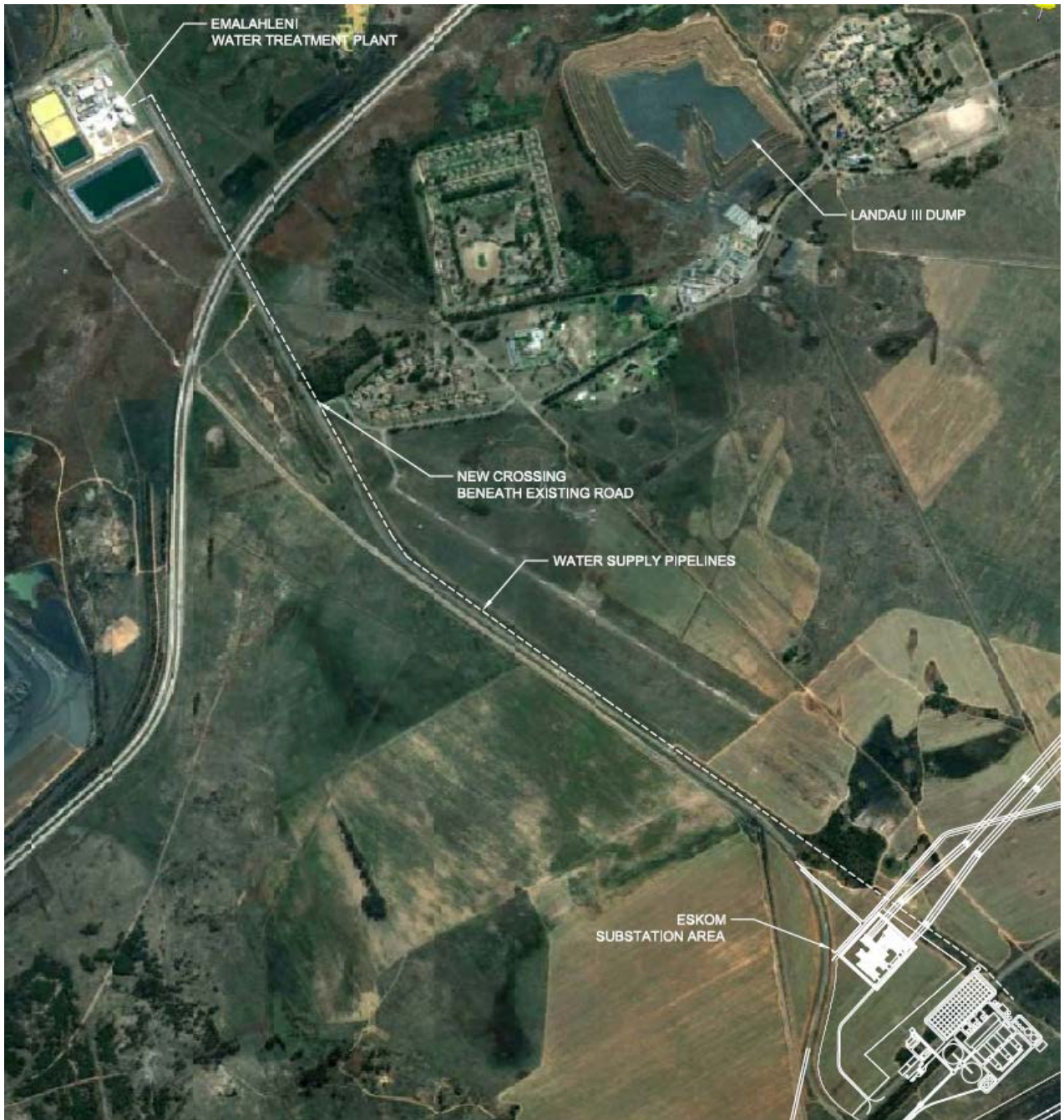
Figure 4-15 Proposed water pipeline route from EWRP
