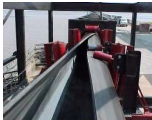
Figure 3-11: A pipe conveyor closing over 10
