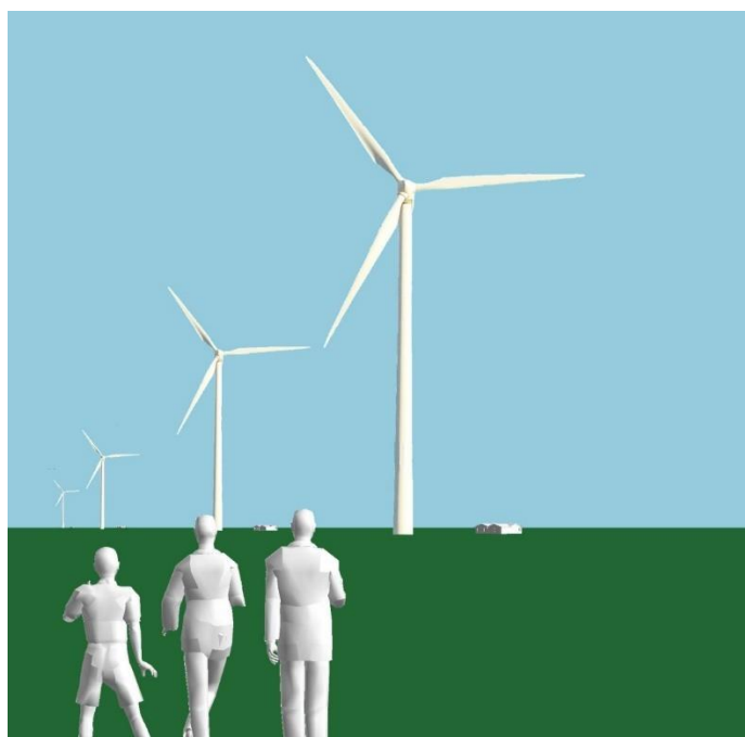
Figure 12: Schematic representation of a wind turbine from 1, 2, 5 and 10km under perfect viewing conditions.
