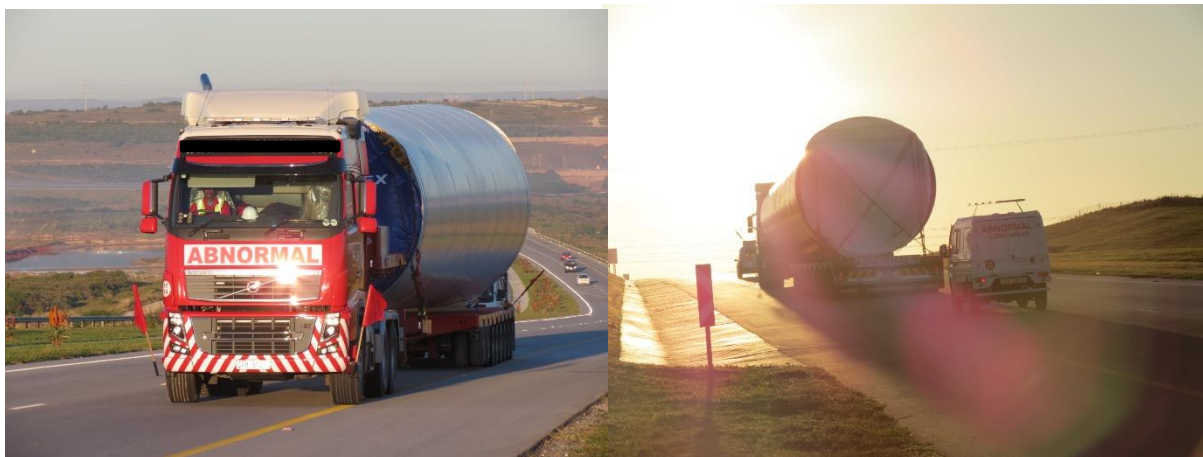
Figure 2-4: Example – Transportation of Tower Sections
