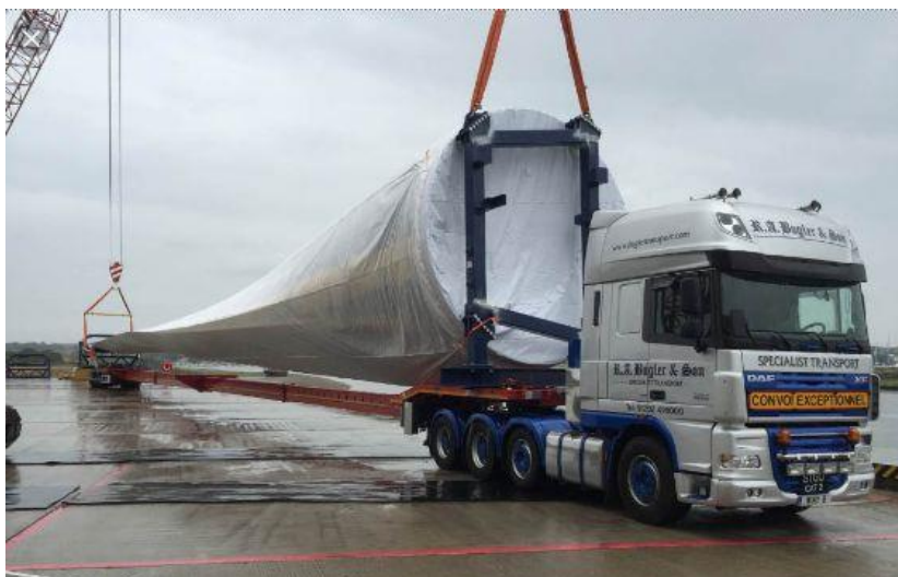
Figure 2-2: Example -Transport of Blades on extendible trailers
