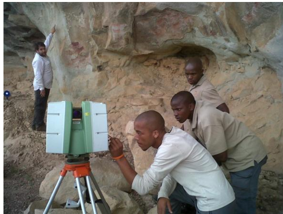
Land surveyors from the RAMP project receiving training by Justin Barton from CyArk in the 3D scanning of rock art.
