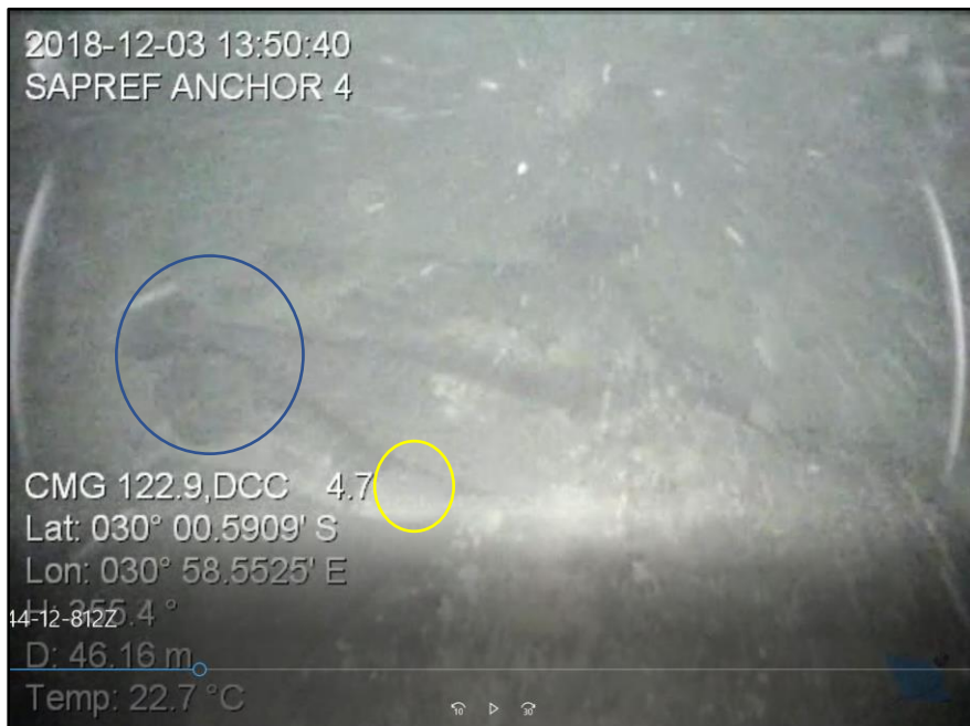
Figure 2: Metal plating is visible, with thickened edges (yellow) as well as standing rigging (blue)
