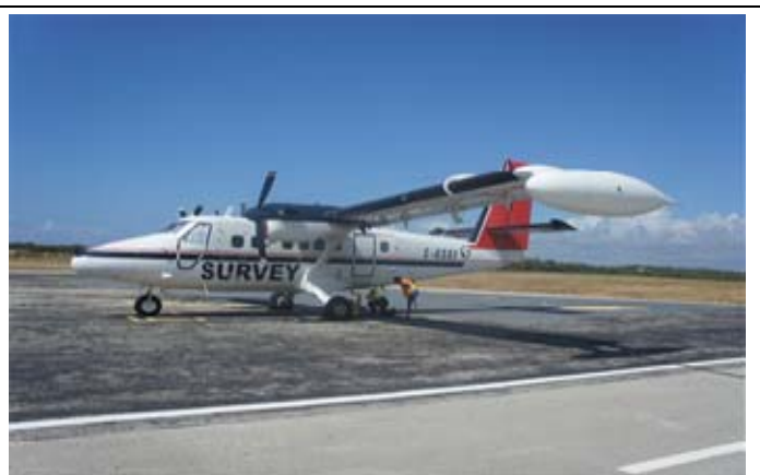
Figure 8: Typical survey plane
