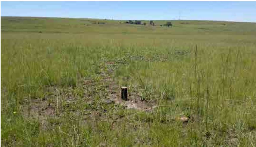
FIGURE 4-14: COMPLETED EXPLORATION BOREHOLE (STAND PIPE STILL TO BE CUT BELOW GROUND LEVEL)
