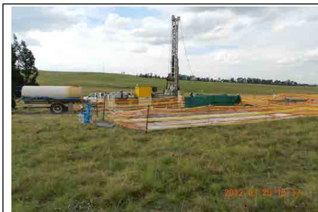
Figure 4: Typical core borehole drilling rig
