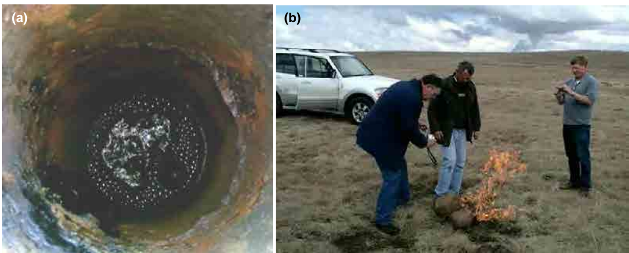
FIGURE 4-4: HISTORICAL COAL BOREHOLE: (A) GAS BUBBLING OUT THROUGH WATER; AND (B) METHANE GAS BURNING WHEN IGNITED
