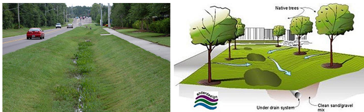
Figure 5.3: Examples of grass swales which can be implemented on low gradient areas within the site. Left image was extracted from Jaxshells (2019), whilst the right image was extracted from WBDG (2016).
