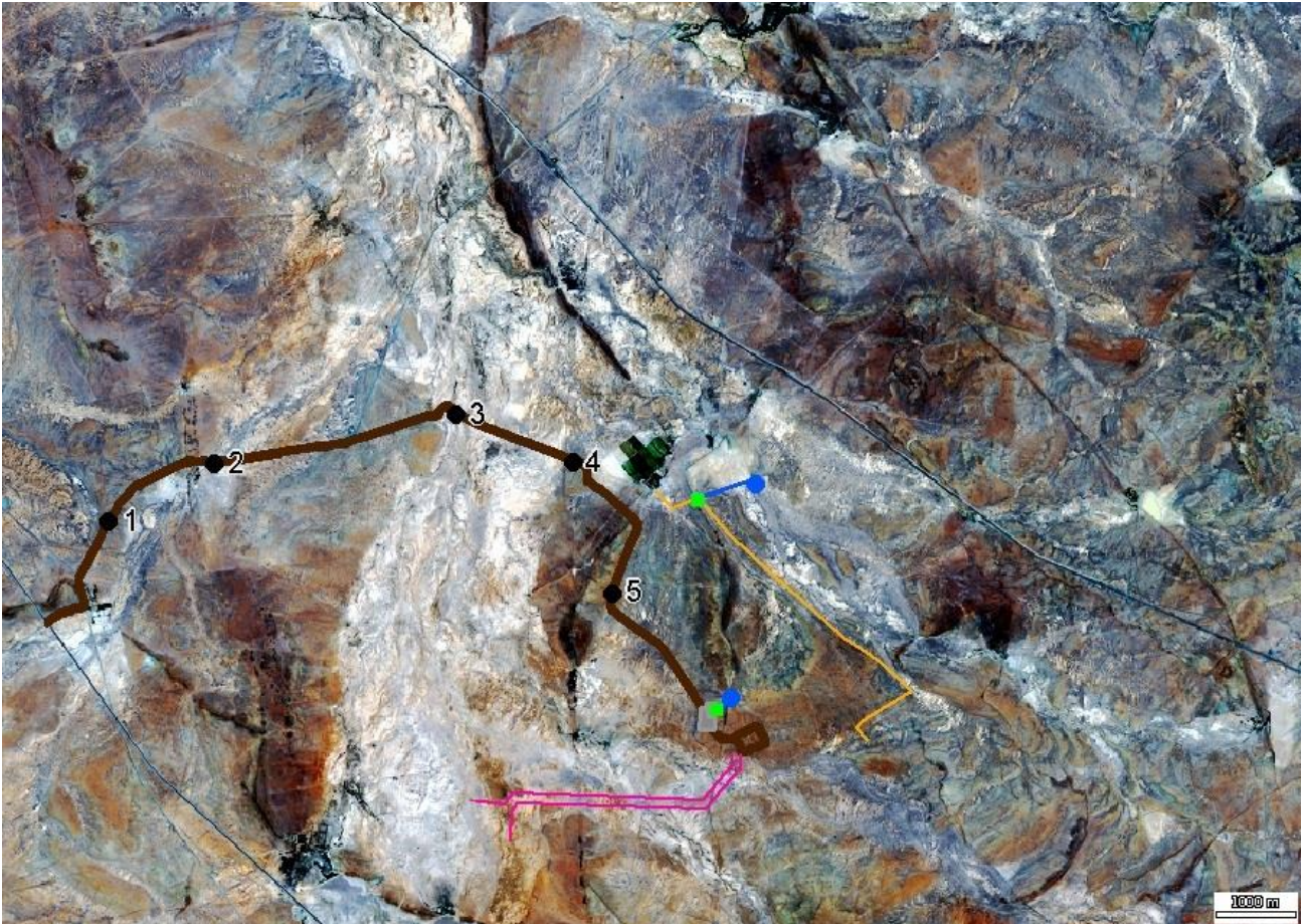
Figure 1. The access road (dark brown with black soil sampling sites no 1-5) to the MTS, water pipelines (blue), boreholes (blue dots), water storage (green squares), temporary construction yard + O&M offices (grey block), 11 kV power line (orange) and 400 kV transmission lines (purple) overlaid on a Sentinel satellite image (2020 12 20).
