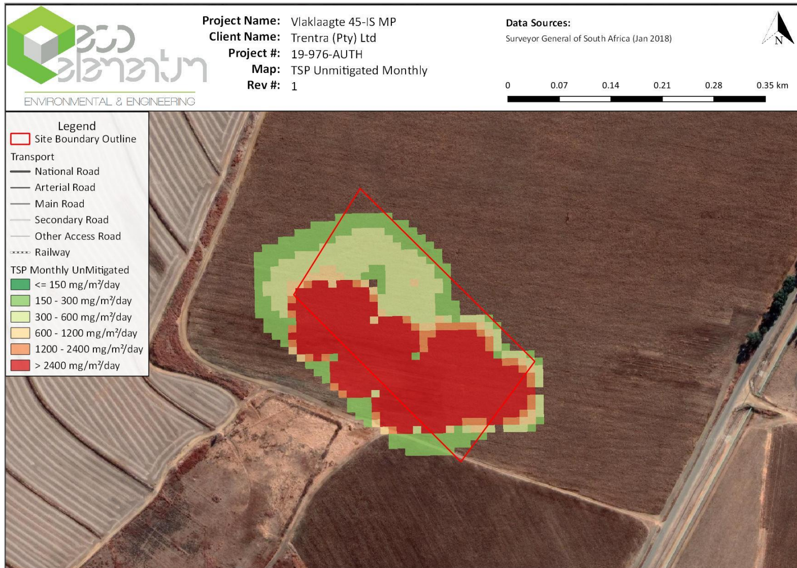
Figure 28: Predicted highest monthly deposition for TSP for the proposed Vlaklaagte project operations when unmitigated.
