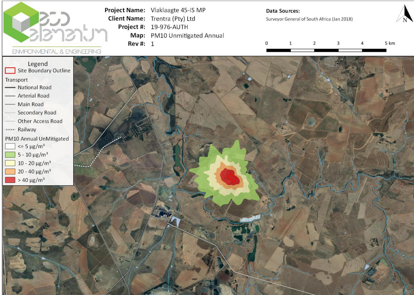
Figure 22: Predicted average annual concentrations for PM10 for the proposed Vlaklaagte project when unmitigated.
