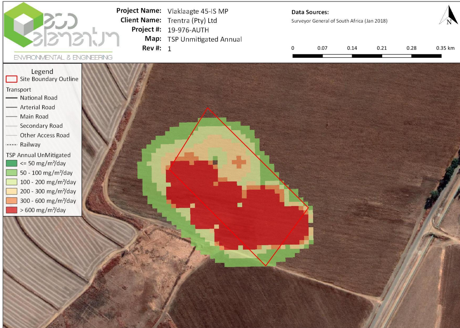
Figure 26: Predicted average annual deposition for TSP for the proposed Vlaklaagte project operations when unmitigated.
