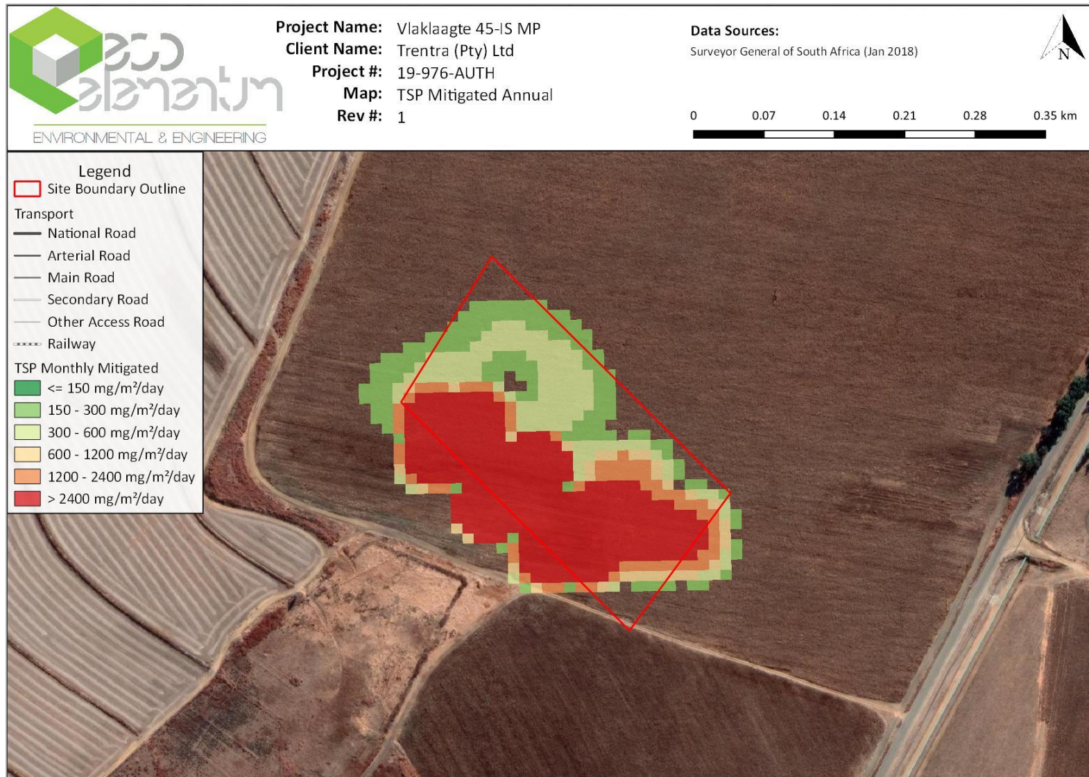
Figure 27: Predicted average annual deposition for TSP for the proposed Vlaklaagte project operations when mitigated.
