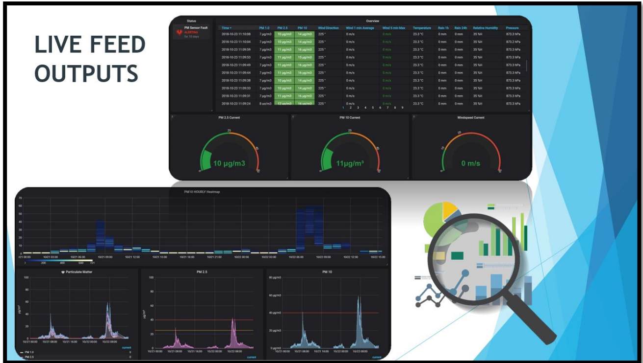
Figure 16: Typical Real-Time Ambient Particulate Matter monitoring dashboard communication interface
