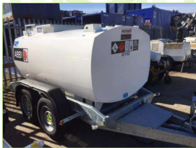
Figure 65: Typical mobile fuel storage trailer with bunded tray
