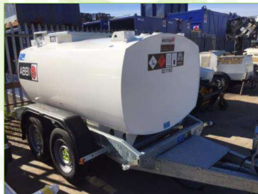
Figure 14: Typical mobile fuel storage trailer with bunded tray
