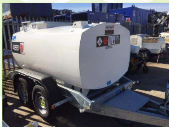
Figure 28: Typical mobile fuel storage trailer with bunded tray
