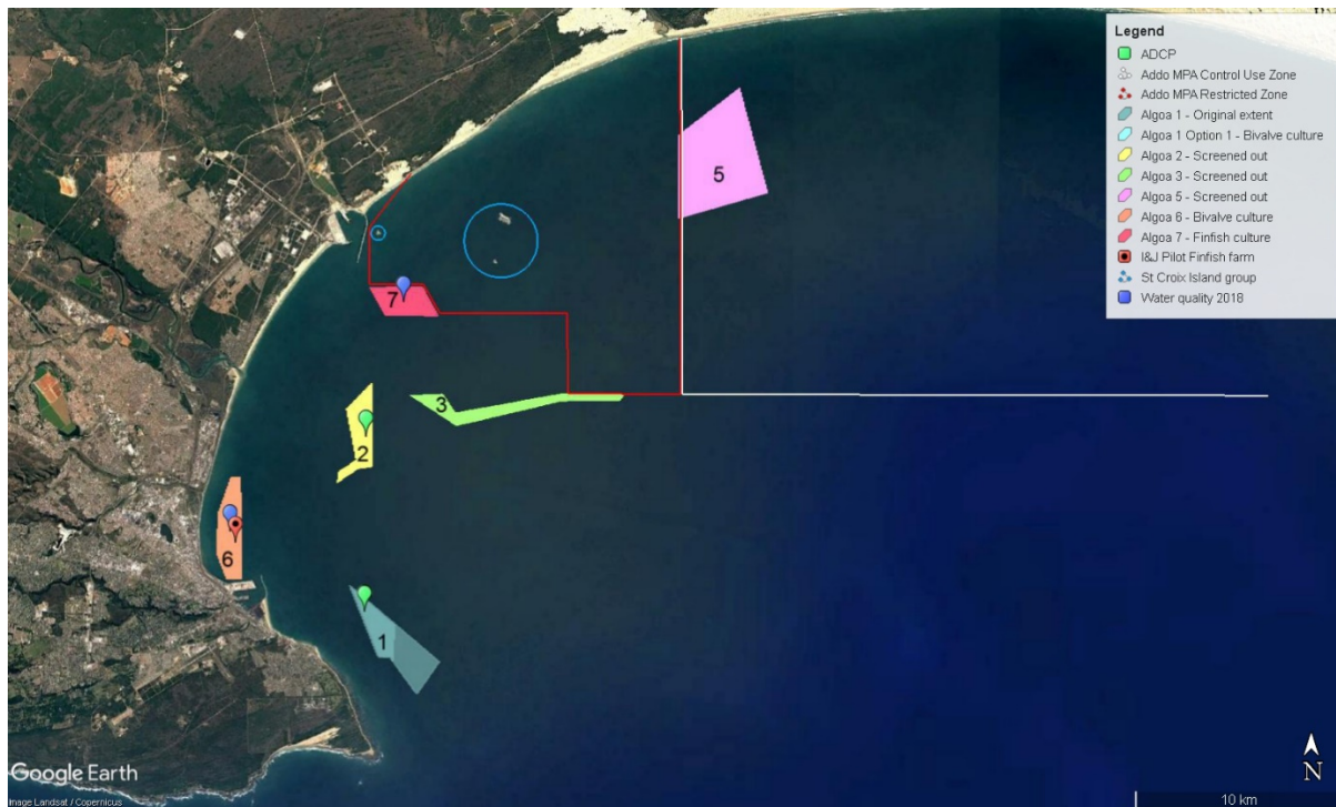
Figure 2 Location of Acoustic Doppler Current Profilers (ADCP) deployed in 2012 over an 11-month period. Data collected at Algoa 2 has been used as a proxy for Algoa 7 precinct. Note that oceanographic data was also collected at Algoa 5 and 3 but have not been included here as the sites have been screened out. Bathymetric surveying was conducted for Algoa 1 (original extent in 2013), as well as for Algoa 6 and 7 (2018).
