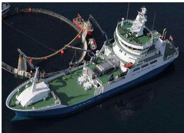
**FIGURE 2. REMOTE FARMS AT EXPOSED SITES MAY BE MAINTAINED BY VESSELS UP TO 40M LONG. (SOURCE: VIELMA AND KANKAINEN, 2013)**
