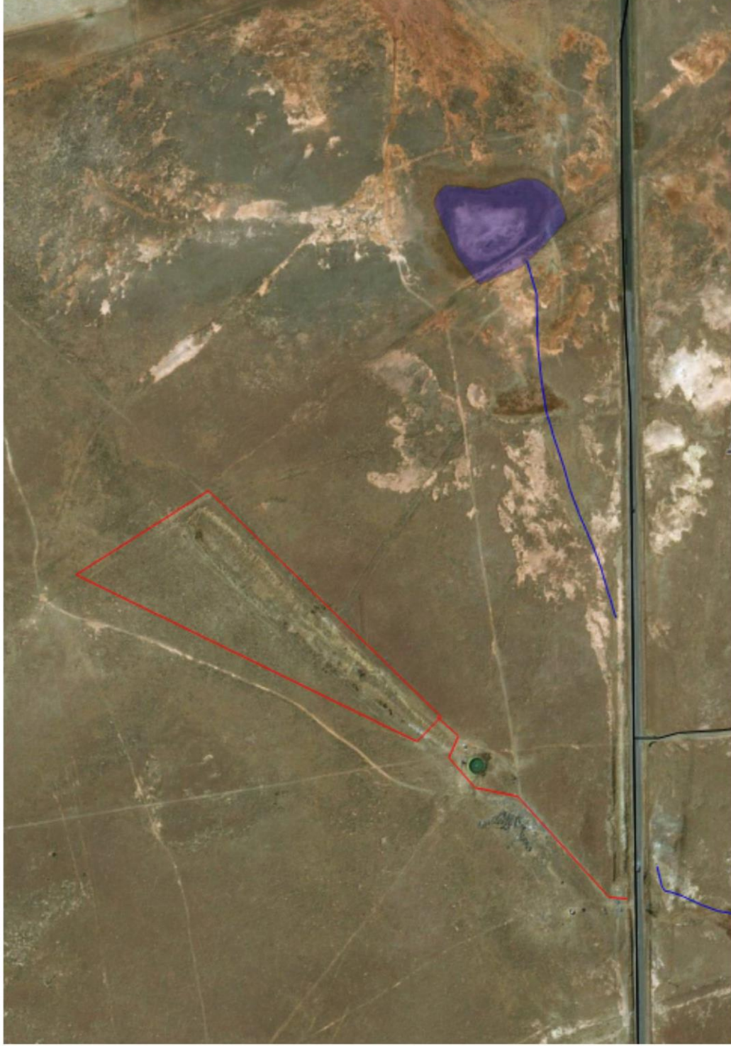
Map 1: Layout map of the proposed borrow pit adjacent to the R58 Provincial Road. The proposed development footprint and access road is indicated. Note that an existing road will be utilised. The existing borrow pit excavation is clearly visible. The surrounding area consists of extensive natural grassland. Note the small drainage line to the south of the proposed borrow pit. It is however not located near the site and prevalent runoff patterns should prevent the development from having any significant impacts on it.
