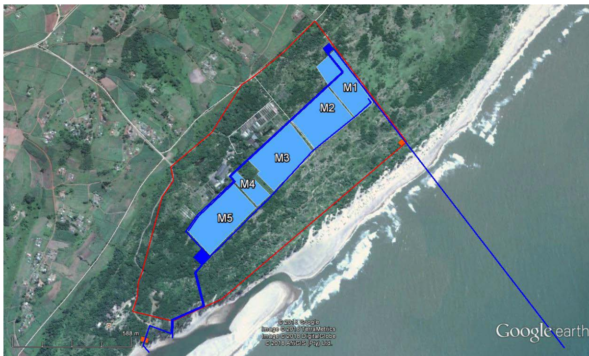
Layout 6: Proposed seawater supply, treatment and discharge for the Amatikulu Aquaculture Development Zone, including estuarine abstraction and discharge.
