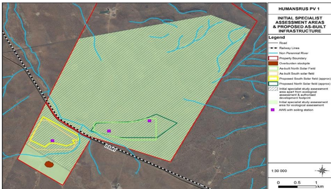
Figure 4: As-built and proposed infrastructure (north and south solar fields with PV arrays, AWS and soiling stations)
