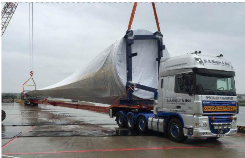
Figure 2-2: Example -Transport of Blades on extendible trailers
