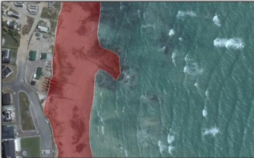
Figure 10: The coastal erosion high risk area highlighted in red.
