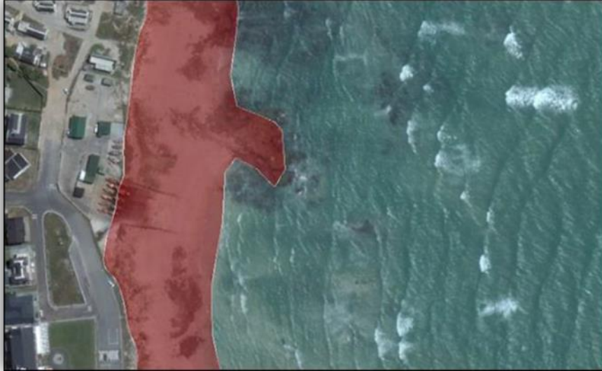
Figure 2: Arniston harbour – coastal erosion high risk area highlighted in red.
