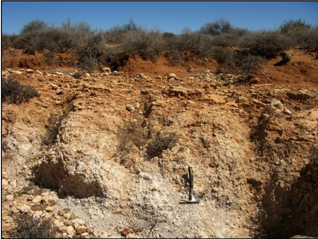
Fig. 16. Quarry face on the south-eastern edge of Q1 showing thick calcrete hardpan, denser towards the upper surface, overlain by downwasted or stream-reworked gravel horizon and orange-brown soils (Hammer = 30 cm).
