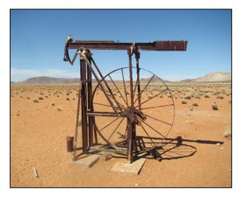
*Figure 23:* The pumping mechanism with the plugged borehole at lower left.
